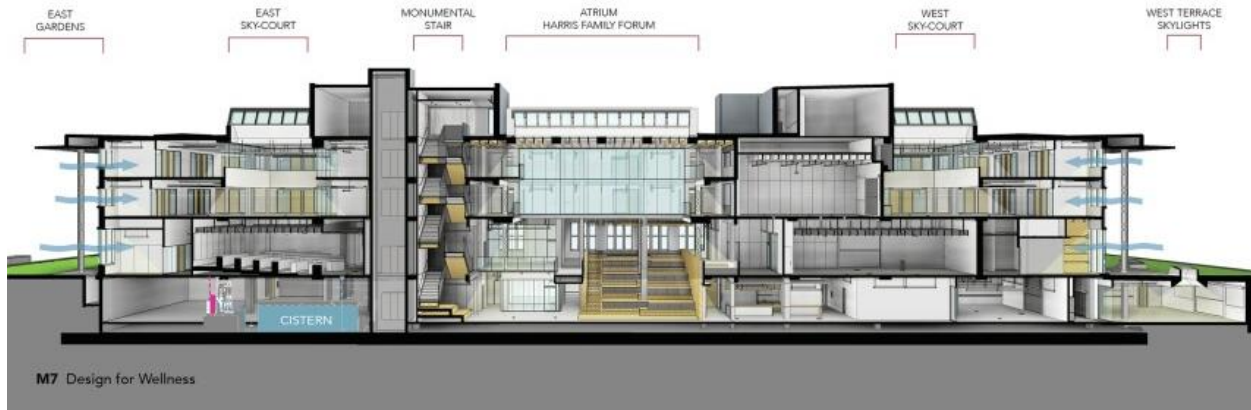
Fig. 5.2 – Raising the ceilings and opening up the building to incorporate more natural light https://www.aia.org/showcases/6280257-keller-center---harris-school-of-public-po
