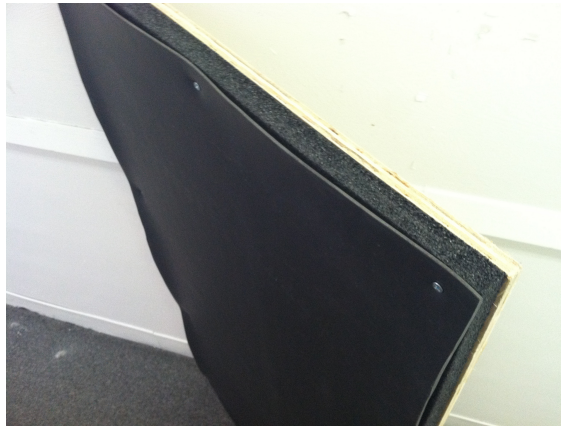
Figure 20: Partition model and final design. All three layers of material and the screws used to secure them are visible.
