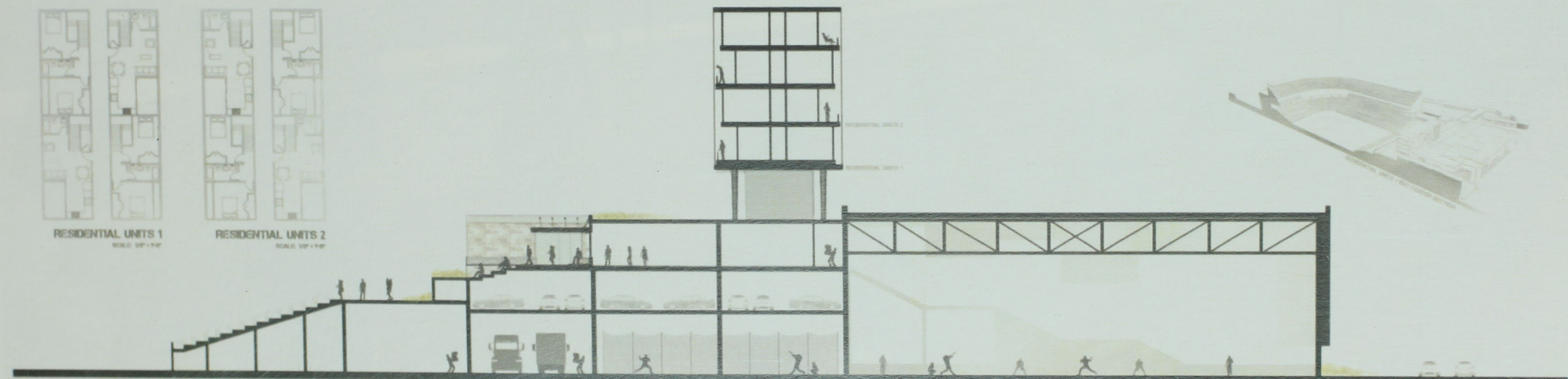
RESIDENTIAL UNITS / REC CENTER SECTION SCALE: 1/8" = 1'-0"
