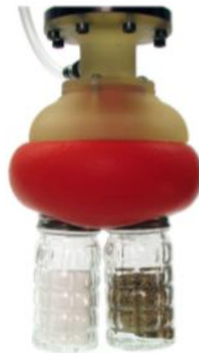
Fig. 1. A universal jamming gripper is able to grip a wide variety of objects without grasp planning or sensory feedback. Multiple objects can be gripped at once, as demonstrated here with salt and pepper shakers.
