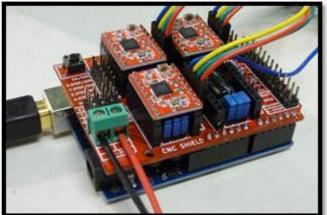
We selected the CNC shield for ease of integration. The premade shield came with drivers, allowing us to skip the guesswork of buying components individually. Additionally this made the programming to move the motors much simpler. It also makes connecting power and other wires much easier with the screw terminals.
