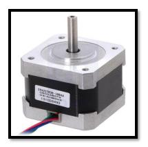
Arduino "brain" using readily available stepper drivers. Additionally these stepper motors offered us an amazing tolerance on our feed length. These motors are capable of moving in 1.8 degree increments that allows us to adjust our wire length down to approximately .030" increments.
