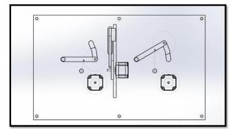
mounted to an arm on spring-loaded pivot allowing the rollers to apply compressive forces to ensure there is adequate friction to pull and drive the wire.
