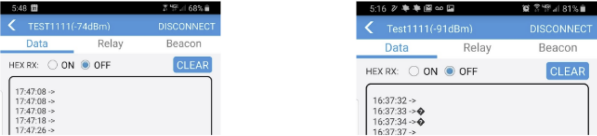
Screen shots showing a clear attenuation increase. Left figure captured when no hand was present. Right figure was recorded with a human hand present.
