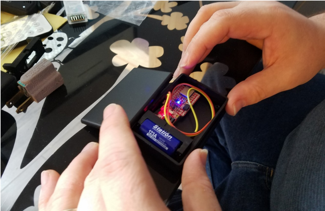
Assembling the SparkFun primary module. Resistors and thermistor have been soldered to the underside of the board.
