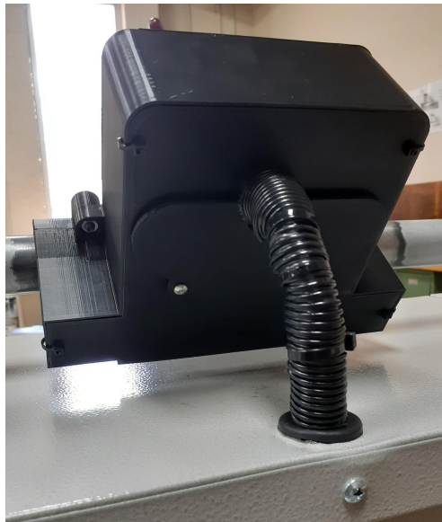
Figure 25: Control Housing Wire Path
