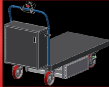
Powered Cart Design based on Manual Cart Platform
