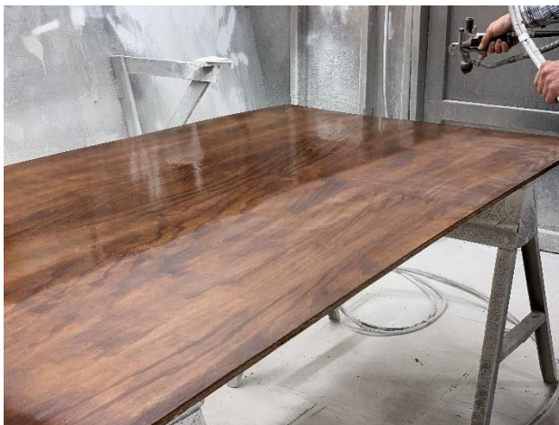
Figure 20: Finishing the Plywood Top
