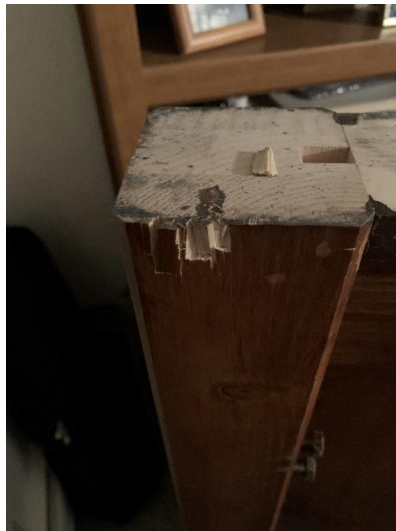
Figure 26: Second Damaged Footboard Leg
