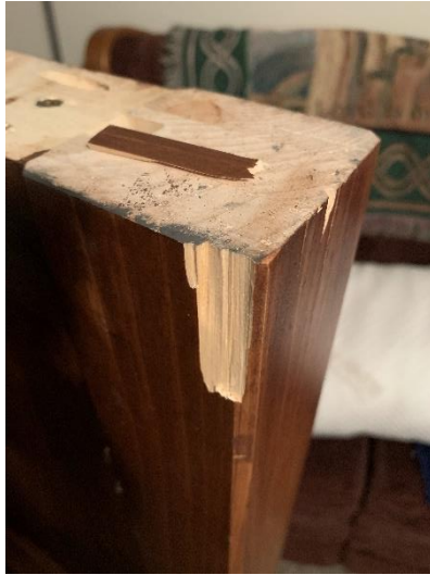
Figure 23: Damaged Footboard Leg
