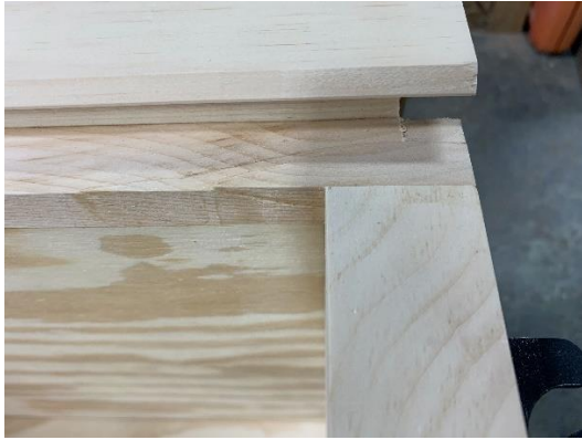
Figure 18: Fixed Face Frame After Crack
