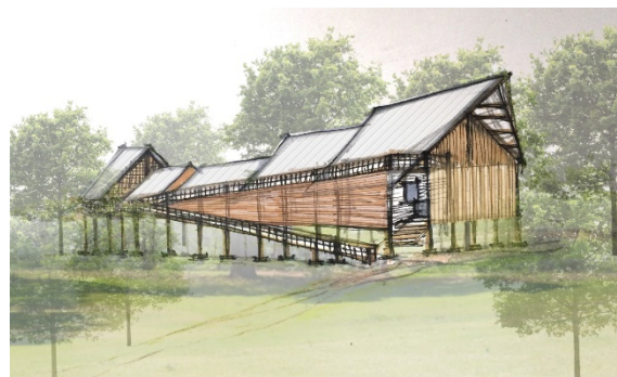
Fig 25: Overhanging roof on the west side; illustrated by author.
